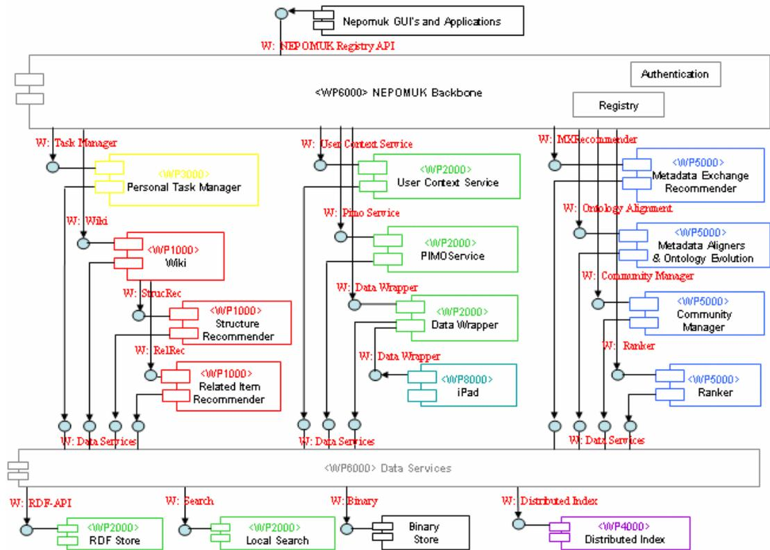
Figure 7. Current NEPOMUK Component Architecture Diagram
